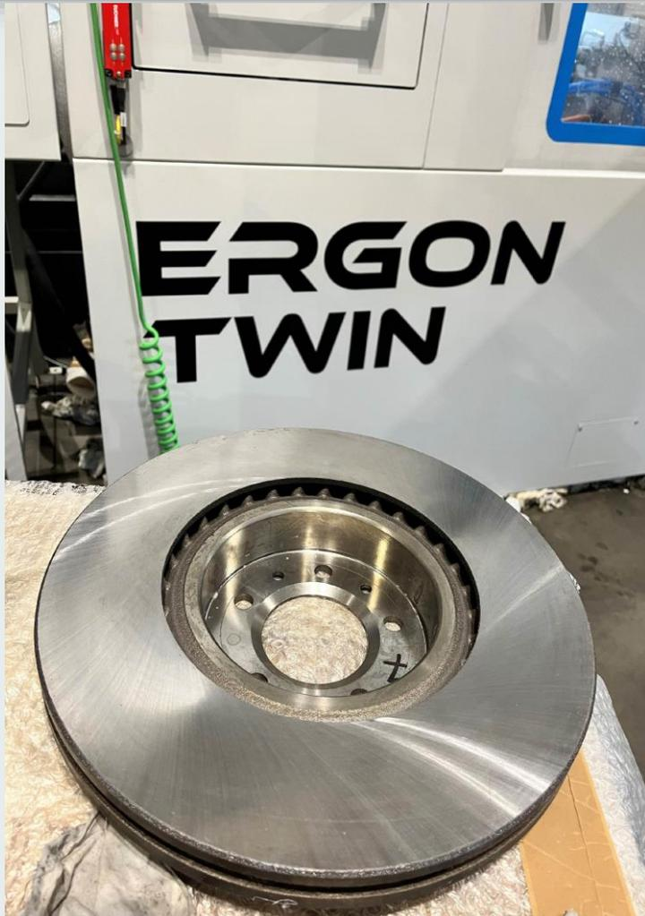
The machine under consideration, follows this philosophy of double working station, and is designed for the grinding of the tracks of brake discs in titanium carbide with different dimensions.
