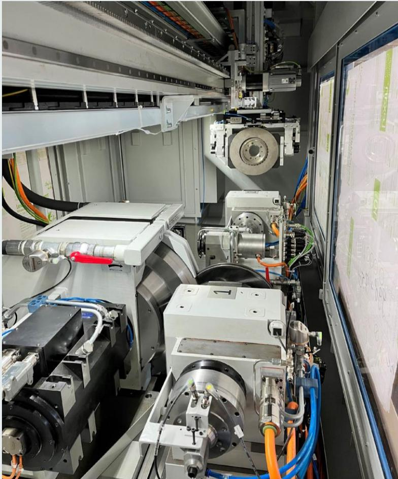
The most characteristic use of Ergon twin to date is the possibility of adding to the double cross axes, a double work station, all served by a loading and unloading system integrated in the machine so as to avoid projections of fog on the outside.
