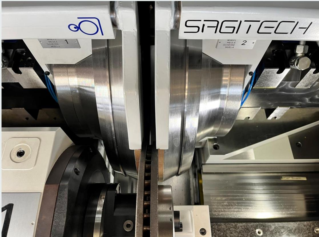
The lubrication of the grinding wheel is in fact carried out with a particular system, result of many studies, that, thanks to the shape of the coolant supply chamber, the shape of the grinding wheel support and the shape of the cooling nozzle, recovers the liquid sent between grinding wheel and workpiece and, by means of a centrifuge system, which creates a vortex, re-sends the same on the contact part grinding wheel/workpiece.
