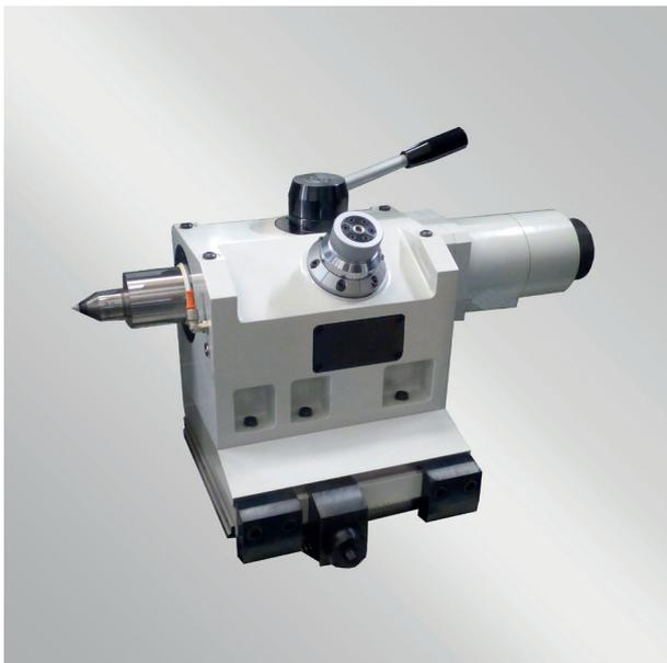
The **ERGON** tailstock unit has everything you need: movement manually controlled by lever or automatically by pedal; the centre pressure can be adjusted by spring or hydraulic force. The cylindricity correction of the pieces is made by a practical knob equipped with an optical scale. The movement of the group along the table takes place through a rack that facilitates the operator in the setup operations.
